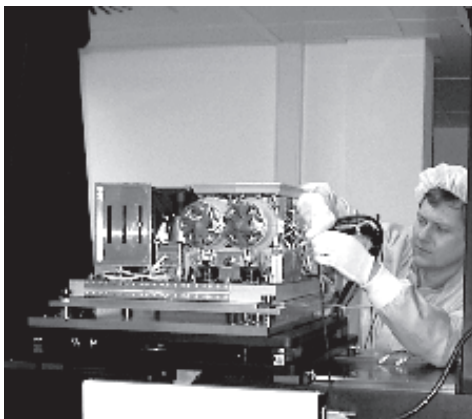
Fig. 2: BIRD payload platform with instruments at the calibration facility.
