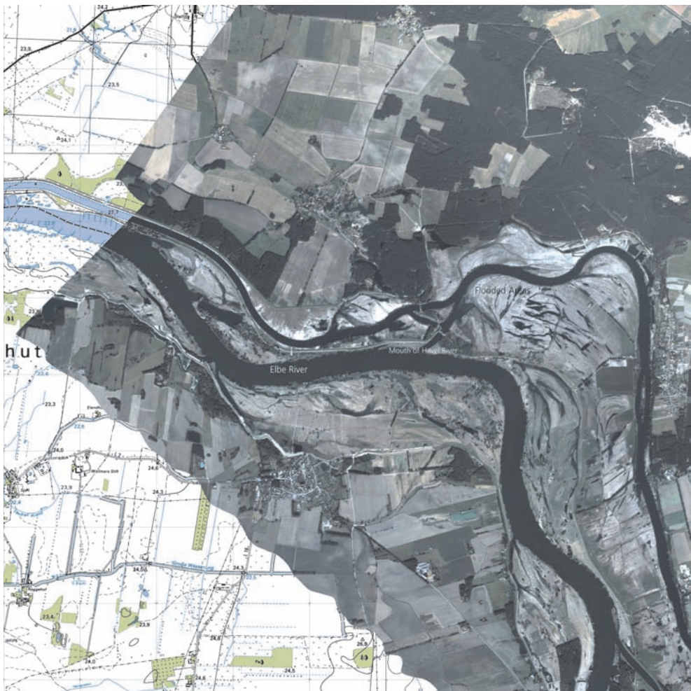
Fig. 4: Part of an orthoimage mosaic (3flight stripes) of the rivers Elbe and Havel about two weeks after the heavy floodings in August 2002, integrated into a topographic map.
