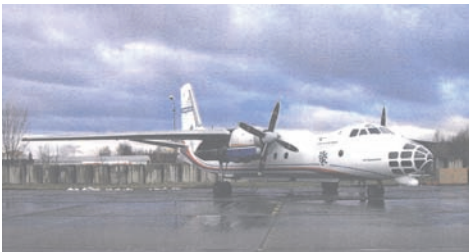
Fig. 4: FOTOLET Antonov AN-30 survey aircraft in service since 1988, painted for OPEN SKIES operations. Mission planning and guidance is done by IGIs WWMP and CCNS4 .
