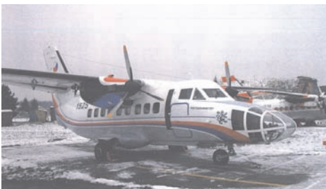
Fig. 5: Let L-410 FG survey aircraft, in operations with FOTOLET since 1985. Mission planning and guidance is done by IGIs WWMP and CCNS4 .
