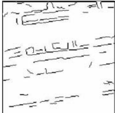
(b) Edge pixels with high gradient magnitude
