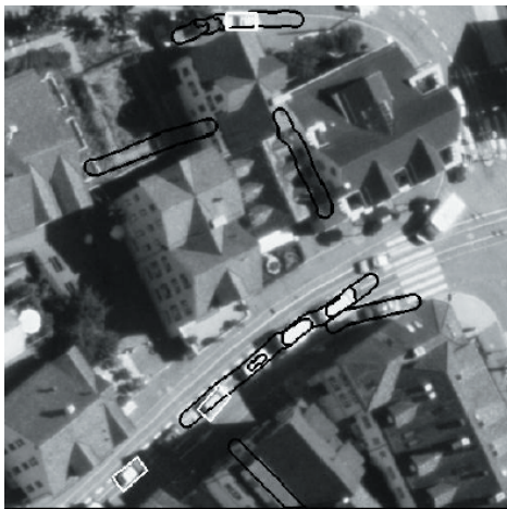
(a) Vehicle detection (white), queue, and blob detection (black)
