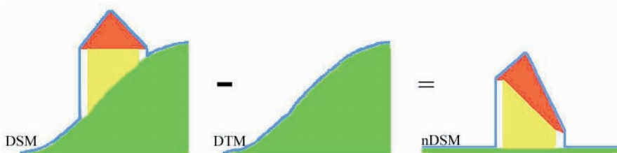
Fig. 1: Problem building case on nDSM.
