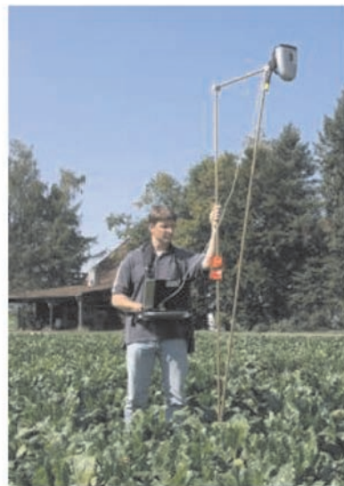
Fig. 1: Designed measurement device for collecting hyperspectral field data.
