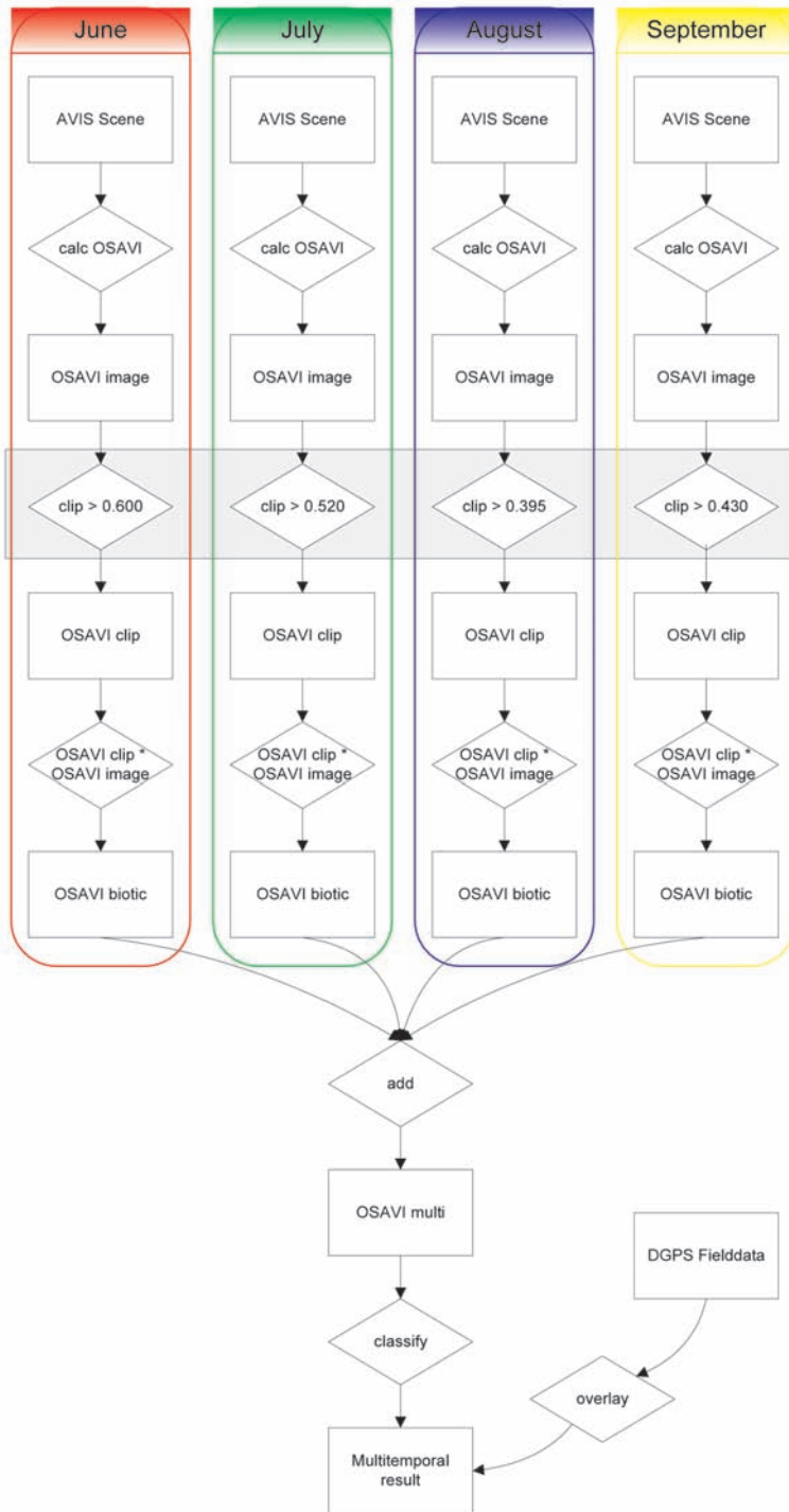
Fig. 2: Knowledge based multitemporal analysis method (note: the threshold values of the clip procedures are chosen out of Tab. 1, figure = exemplarily for the AVIS data) (LAUDIEN et al. 2004c).
