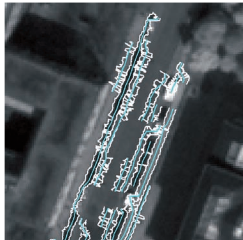
Fig. 5: Width extracted from gradient image: Extracted edges (white), queues' control lines (cyan).
