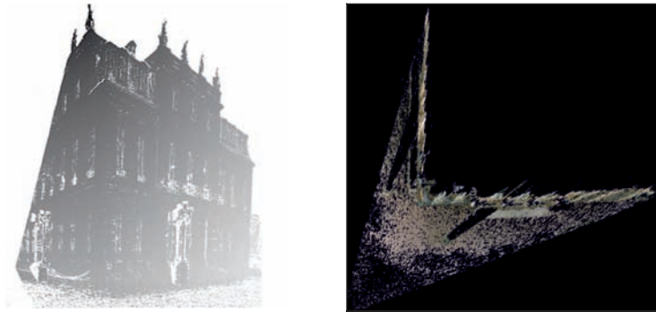
Fig. 5: a) The resulting disparity map of the Stuttgart palace using the modified SGM and b) top-view on the point cloud of the reconstructed corner.
