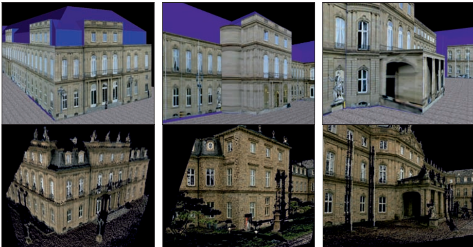
Fig. 6: Available architecture model of the Stuttgart palace from aerial images improved by manual texture mapping (top) and 3D point clouds acquired automatically with the proposed trifocal sensor system using one image triplet (bottom).
