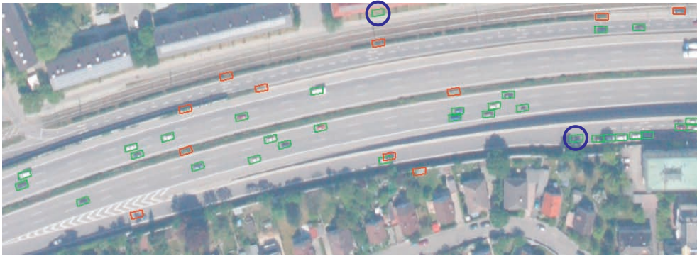
Fig. 10: Refined track results. Green: Detected and tracked vehicles. Red: Eliminated false alarms after velocity evaluation. Blue circle: False alarm which has not been eliminated.
