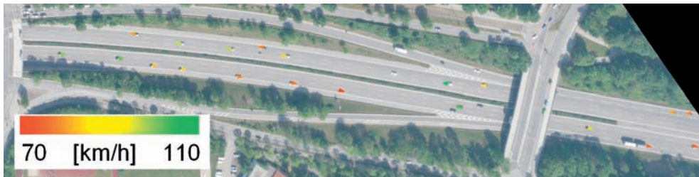
Fig. 7: Resulting velocities of vehicles measured by car tracking.
