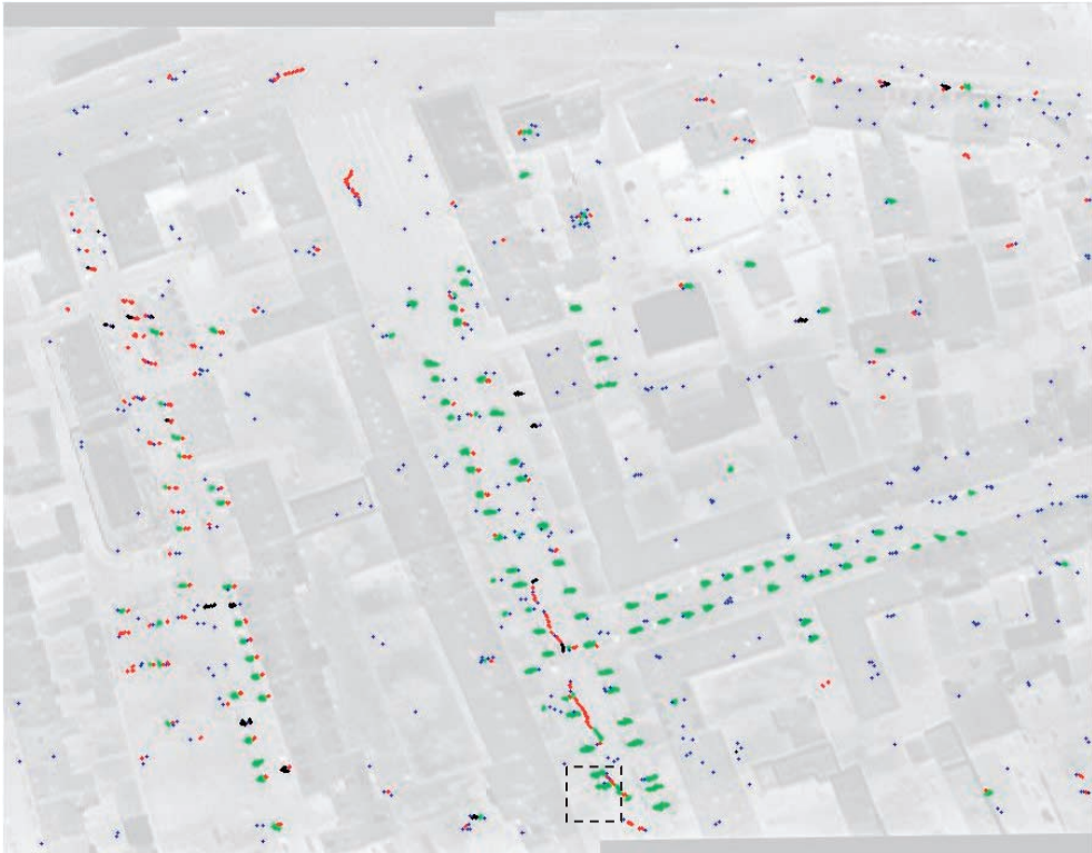
Fig. 6: Vehicle region map after preliminary classification, green: stationary vehicle; blue: single vehicle; red: moving vehicle; black: hybrid vehicle.
