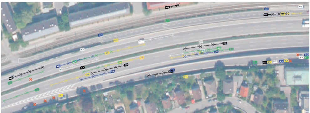
Fig. 9: Results of tracking using image triplets with trajectories of tracked objects. Red crosses indicate detections where the tracking failed.
