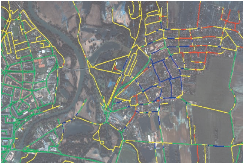
Fig. 9: Detail result of the assessment system using all available input data: image t_1 , image t_2 , DEM and manual generated reference at time t_1 ; green = trafficable, yellow = possibly flooded, red = flooded, dark blue = trafficable (changed from flooded at time point t_1 to trafficable at time point t_2 ).
