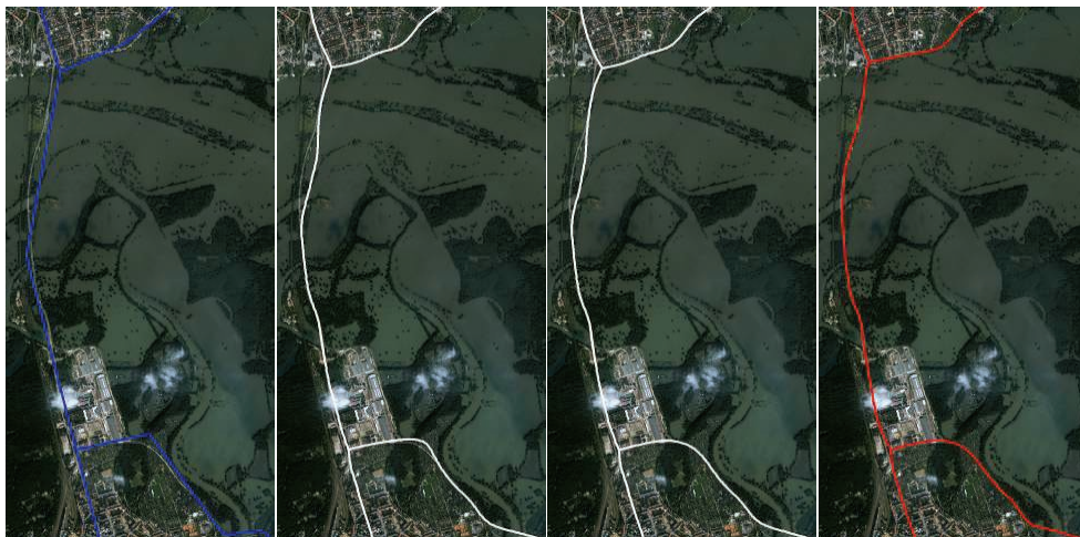
Fig. 6: Automatic road refinement using network snakes in an IKONOS image taken during the Elbe flooding in Germany, 2002: initialization (blue), optimization steps (white), result (red).
