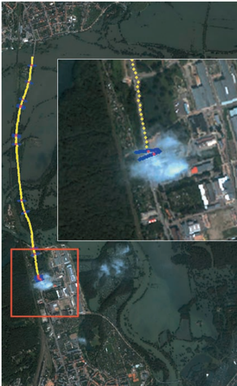
Fig. 5: User-assisted road tracking in an IKONOS image taken during the Elbe flooding in Germany, 2002. Yellow points: tracked road sections; blue lines/red points: user clicks.
