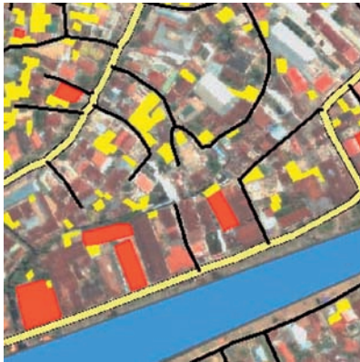
Fig. 14: Reference data, including streets and potentially damaged buildings: red (according to building structure survey) and yellow (on building characteristics derived from satellite imagery).
