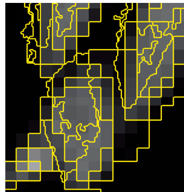
Fig. 3: MRS result using Landsat 7 and TerraSAR-X data – Overlaid on Landsat 7 pre-event scene.
