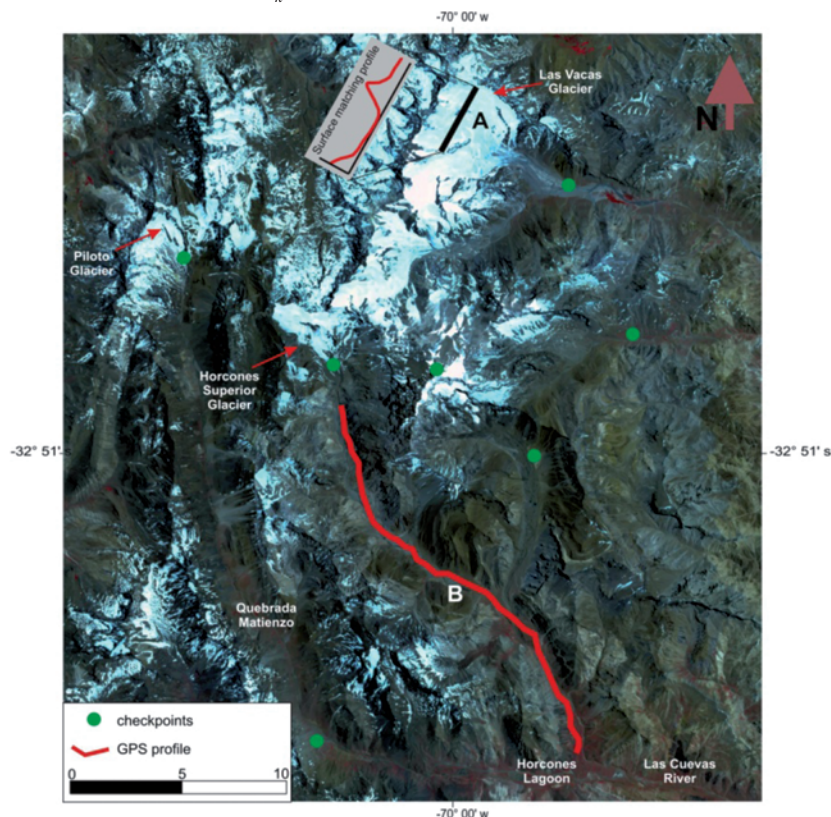
Fig. 5: GPS checkpoints (green) and profile B (red) used for the validation of the DTMs, and profile A (black) used for evaluating the robust surface matching (ASTER image 2001).
