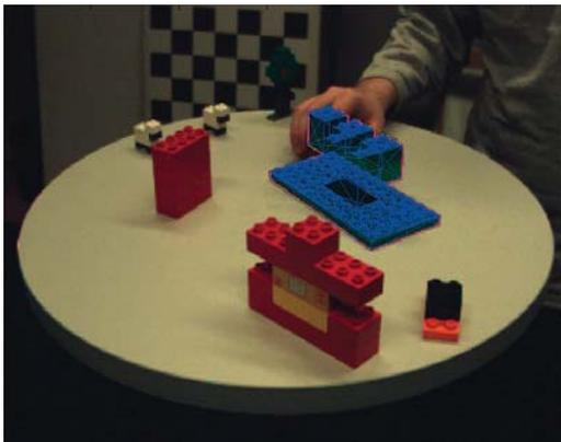
**Fig. 5:** Recursive 3d pose estimation with a single camera of a known object. The object is represented as a meshed shape with observed silhouette points in an image (Image and silhouette data provided by B. ROSENHAHN, MPI).
