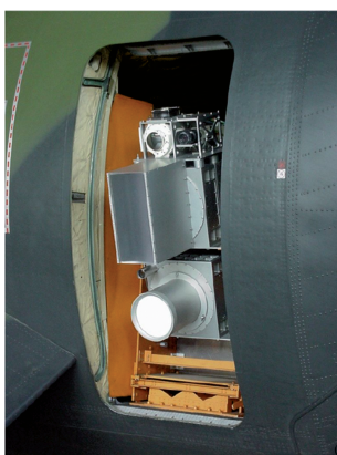
Fig. 2: MEMPHIS radar mounted into a C-160. Top: Synergy infrared optical sensor, center: 35 GHz interferometric SAR antenna with 3^\circ \times 13^\circ beamwidth (box), bottom: 94 GHz polarimetric monopulse antenna with 1^\circ \times 13^\circ beamwidth.
