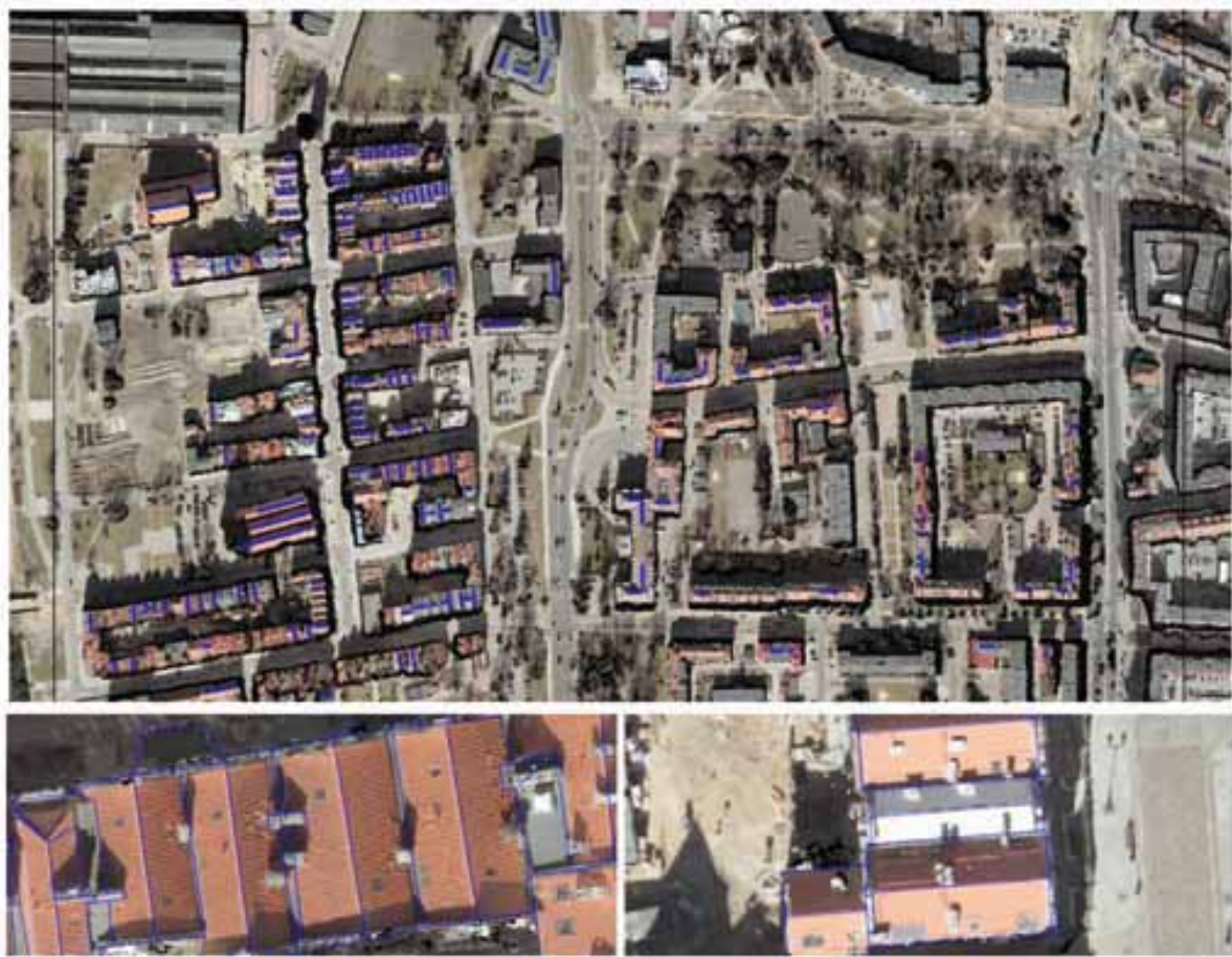
Fig. 4: An overview of all ridge lines extracted from true orthophoto in the test area and a detailed view presenting automatically lidar-extracted building models with true orthophoto from dense image matching in a background.
