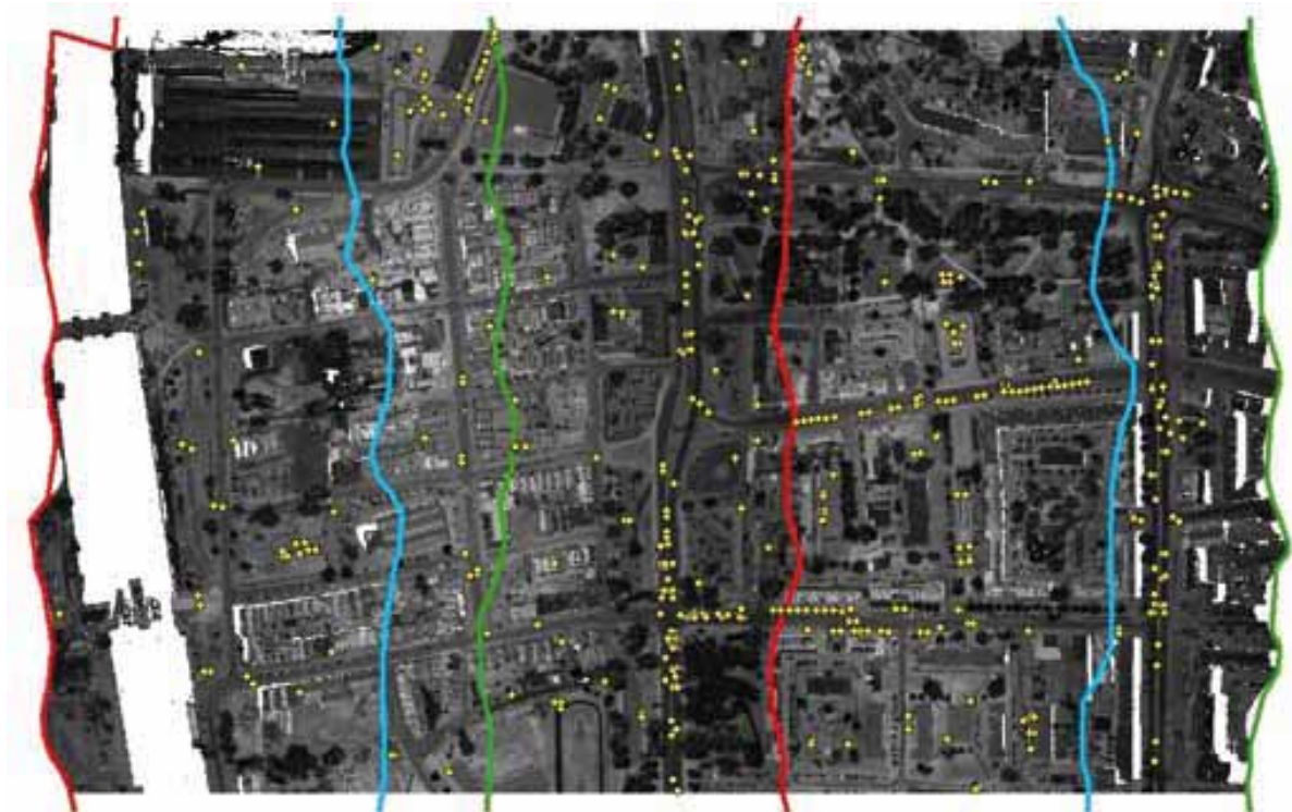
Fig. 1: Spatial distribution of points manually measured on the intensity image and the true orthophoto overlaid with the presentation of the scanning strips edges.
