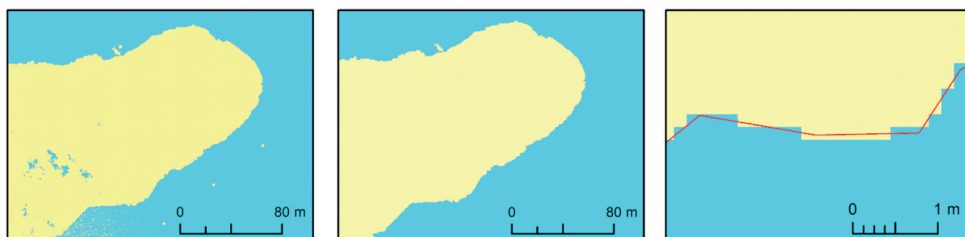
Fig. 5: Left: classified image before the application of morphological operations, middle: classified image after morphological operations, right: vectorized shoreline(subset).
