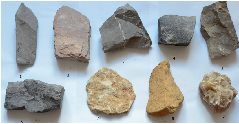
Fig. 6: Samples from the Czatkowice Limestone Mine: microcrystalline limestone (1); weathered limestone (2), (7); silicated limestone (3); bituminous limestone (4), (6); dolomitic limestone (5); sandstone (8); coarse crystalline calcite (9).
