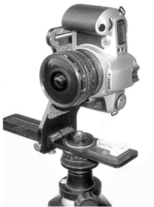
Figure 11: recording of panoramas with a fisheye lens.
