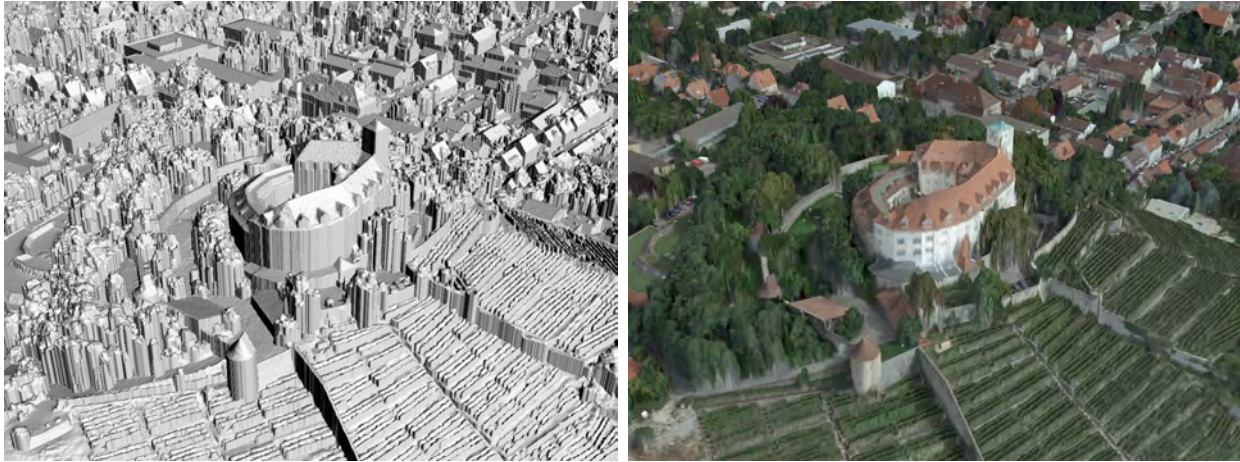
Figure 8: Untextured and automatically textured model from UltraCam-X data set with 8 cm/pixel
