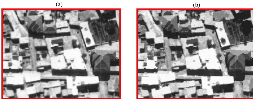
Figure (9): The whole historical image has been enhanced by MDV-based approach; (a): the historical image before the enhancement, (b): the historical image after the enhancement process
