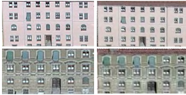
Figure 5: The marked sections of Figure 4 have been rectified. At left are two sections from the oblique data at 45°; at right from the vertical data at 27°.
