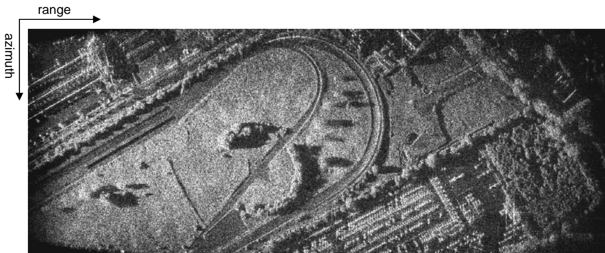
Fig. 4: Image focused with the SPECAN algorithm. The individual RC data bursts are 0.7 s long (or ~22 m flight distance). The focussed image covers a surface of about 310 m in azimuth x 800 m in range.
