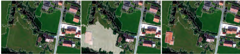
Fig. 7: Segmentation using threshold test and universal segment removal of two scenes with simulated changes and parameters T=75 , T_{\text{check}}=75 ; from left to right: Segmentation of first image using multiresolution segmentation, segmentation adapted to second image after consistency check and segment removal, final segmentation of the second image
