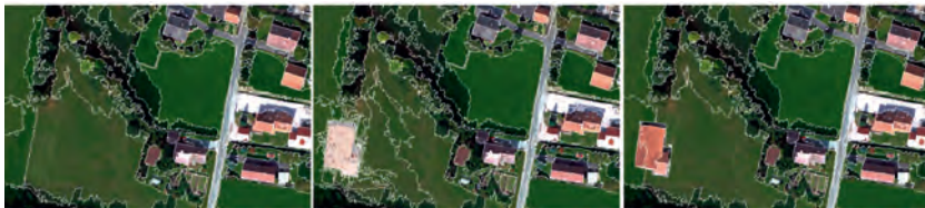
Fig. 9: Segmentation using local best fitting test and local segment removal of two scenes with simulated changes and parameters T=75 , T_{\text{check}}=75 , T_{\text{checktolerance}}=0.5 ; from left to right: Segmentation of first image using multiresolution segmentation, segmentation adapted to second image after consistency check and segment removal, final segmentation of the second image
