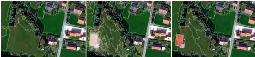
Fig. 8: Segmentation using local mutual best fitting test and global segment removal of two scenes with simulated changes and parameters T=75 , T_{\text{check}}=75 , T_{\text{checktolerance}}=0.5 ; from left to right: Segmentation of first image using multiresolution segmentation, segmentation adapted to second image after consistency check and segment removal, final segmentation of the second image
