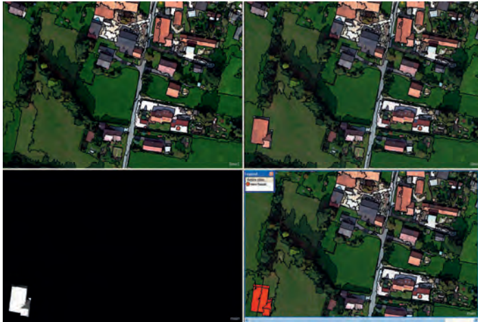
Fig. 10: Result of the change analysis using the method of correspondence via intersection ; from upperupper left to lower right: Segmentation of first image, segmentation of second image, change intensity obtained by MAD, change classification using a threshold
