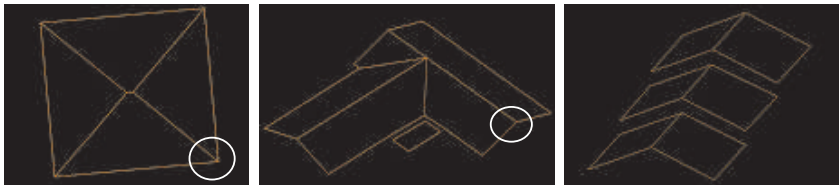
Fig. 7: Sample roof structures: Simple hip roof (left), L-shaped roof with a connected roof by a height jump (middle), Multi-level gable roof (right)
