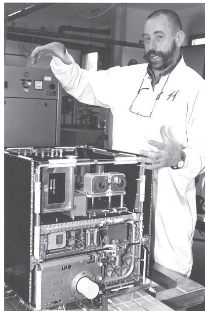
Fig. 3: Structure Thermal Model of the BIRD satellite without MLI.
