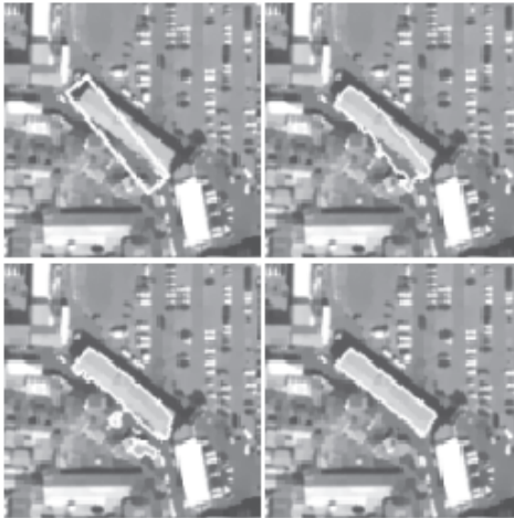
Fig. 5: Convergence sequence (from top to bottom and left to right) illustrating the matching process with a flexible shape constraint ( 5 < \lambda_{flex} < 30 , \lambda_{DSM} = 0 ).
