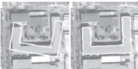
Fig. 3: Matching with shape prior and remote initialization ( \lambda = 10 ). Left: initial state. Right: successful matching result even with remote initialization.
