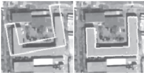
Fig. 6: Matching with DSM fusion ( \lambda_{flex} = cst , \lambda_{DSM} = 0.75 ). Left: initial state. Right: successful matching with DSM fusion.
