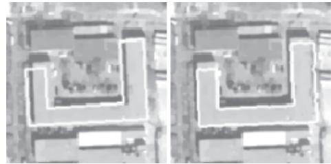
Fig. 8: Matching with flexible shape prior and DSM fusion and a locally mistaken cartographic object ( 5 < \lambda_{flex} < 30 , \lambda_{DSM} = 0.75 ). Left: initial state derived from the map. Right: unsuccessful complete matching result.
