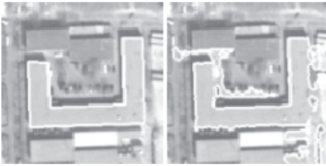
Fig. 2: Matching without shape prior. Left: initial state close to the desired solution. Right: result without shape prior, “leak” of the active contour.
