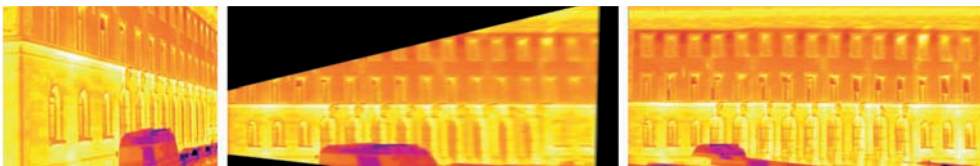
Fig. 4: Steps for generating a single texture: a) IR image, b) extracted single partial texture, c) combined final texture. The color table represents the intensity values of one IR band.
