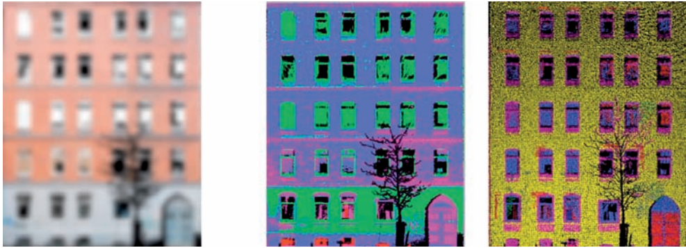
Fig. 4: Smoothed image maintains only large changes in facade structure (left). Clustered facade calculated by colour value and depth (right).
