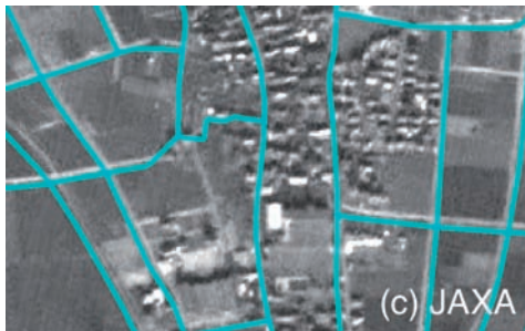
Fig. 2: Typical differences of ALOS PRISM imagery and NTIS road features (light blue).
