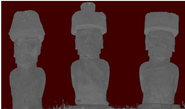
Fig. 5: Representation of point cloud with intensity values, which were scanned from one scanner station at Ahu Nau Nau with the terrestrial laser scanning system Z+F IMAGER 5006.
