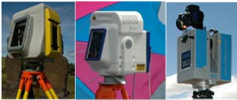
Fig. 1: Terrestrial laser scanner Trimble GX (used in 2007), Trimble GS101, IMAGER 5006 from Zoller & Fröhlich (both used in 2008).
