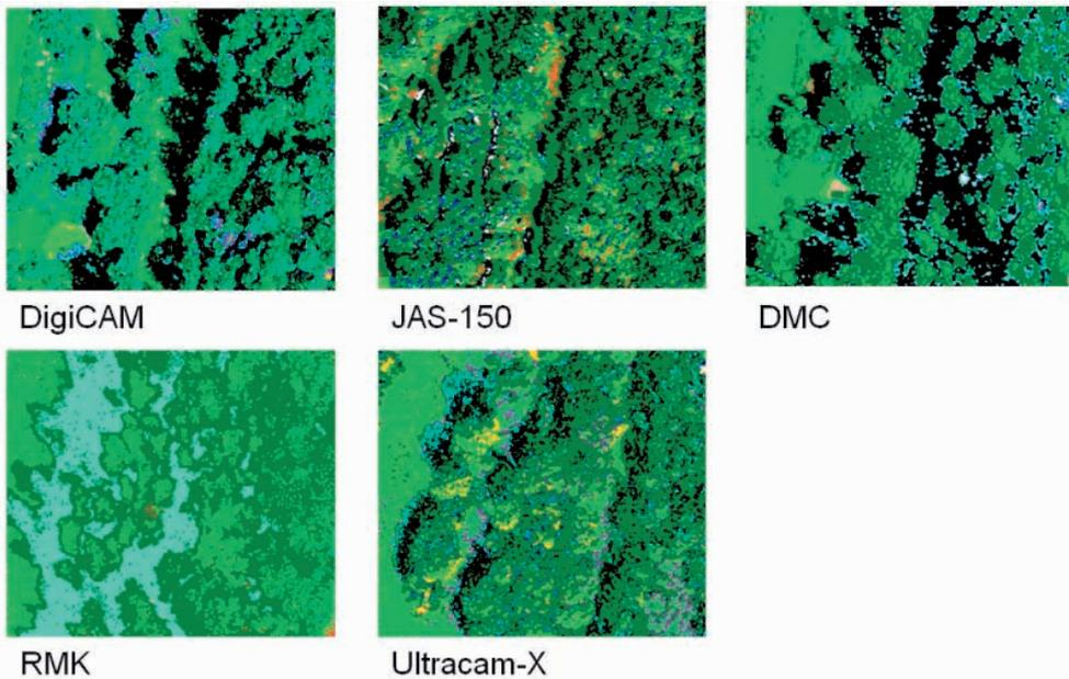
**Fig. 3:** Class “shadow” (for more explanations see KLONUS 2009), obtained from the data sets of the DGPF-evaluation project. The differences result on the one hand from the various properties of the cameras and on the other hand from the different weather conditions.
