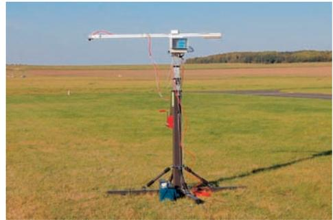
**Fig. 5:** BRDF-instrument GRADIS in operation.
