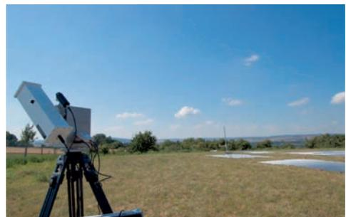
**Fig. 6:** Sun photometer on the test site at Vaihingen/Enz.
