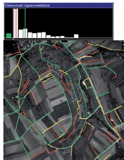
**Fig. 3:** Overview of self-diagnosis. Top: Length-weighted histogram of evaluation scores (left-most bar indicates mean value = green in this example), thin vertical lines indicate thresholds between categories. Bottom: Overview window.
