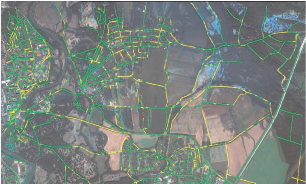
**Fig. 10:** Evaluation of the assessment system using image  $t_2$ , image  $t_1$  and DEM; green = 'correct assignment', yellow = 'manual control necessary', cyan = 'possibly correct assignment', red = 'wrong assignment' [system = trafficable, reference = flooded], dark blue = 'wrong assignment' [system = flooded, reference = trafficable].
