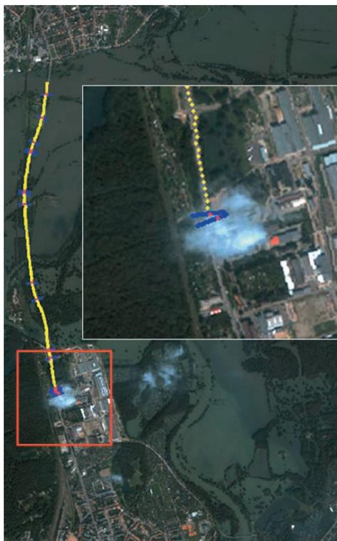
**Fig. 5:** User-assisted road tracking in an IKONOS image taken during the Elbe flooding in Germany, 2002. Yellow points: tracked road sections; blue lines/red points: user clicks.
