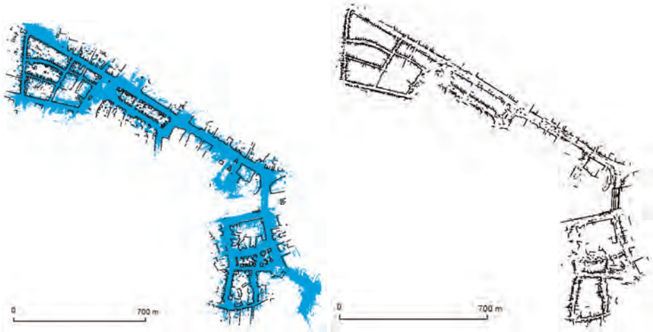
Fig. 3: Building outlines and building facades represented in different data sets. Left: visible digital cadastral map (black lines) with area covered by mobile laser scanning point cloud (blue area). Right: facades extracted from mobile laser scanning data.
