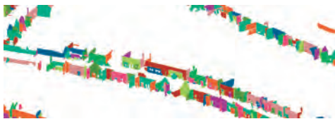
Fig. 7: Extracted laser echoes of facade segments from mobile laser scanning coloured by segment.
