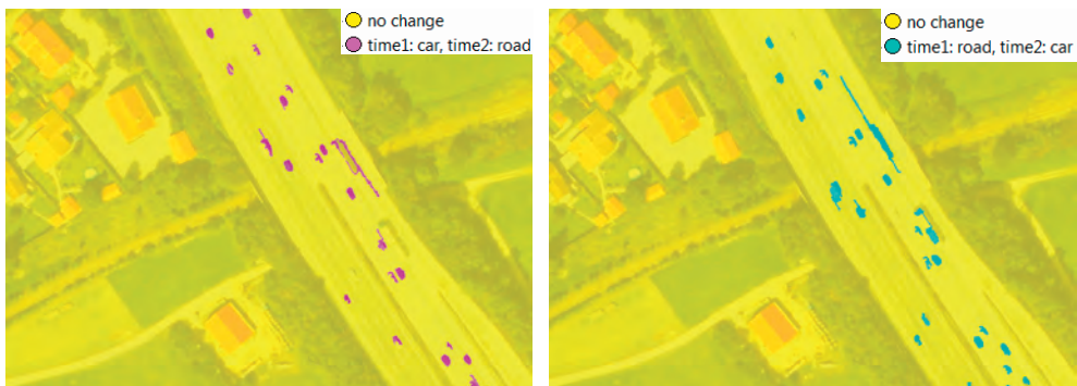
Fig. 7: Directed change detection. Changes from time 1 to time 2 (left) and from time 2 to time 1 (right).
