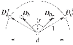
Fig. 3: Enforcing the Plücker constraint onto a 6-vector \mathbf{L}^r = [\mathbf{L}_h^r; \mathbf{L}_0^r] . Starting from vectors \mathbf{D}_h^r = \mathbf{N}(\mathbf{L}_h^r) and \mathbf{D}_0^r = \mathbf{N}(\mathbf{L}_0^r) , which in general are not perpendicular, we easily can enforce the perpendicularity by symmetric linear interpolation, leading to \mathbf{D}_h and \mathbf{D}_0 , which are perpendicular. The vector \mathbf{M} = \mathbf{N}([\mathbf{L}_h | \mathbf{D}_h; | \mathbf{L}_0 | \mathbf{D}_0]) yields a valid Plücker vector close to \mathbf{L}^r .
