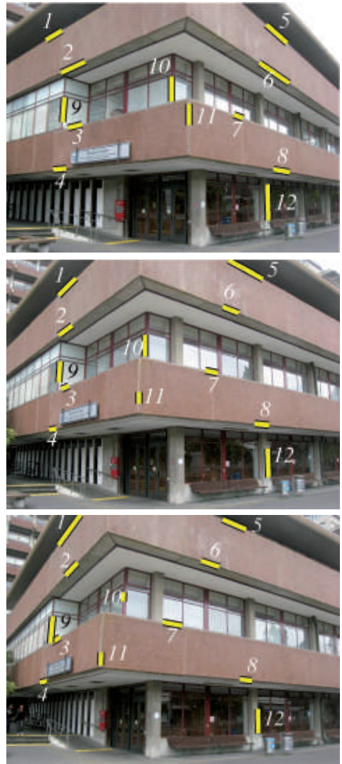
Fig. 4: Three images with 12 corresponding straight line segments used for the reconstruction of the 3D lines, forming three groups [1...4], [5...8], [9...12] for three main directions.
