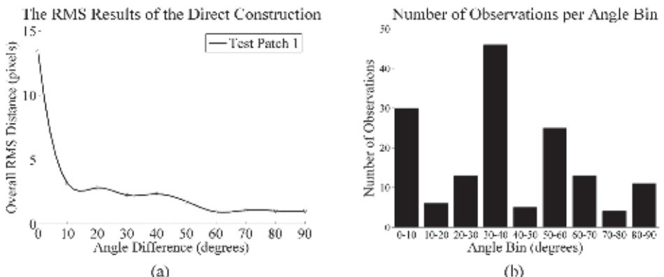
**Fig. 2:** (a) The performance of the direct construction method for various angle differences ( $0^\circ$ – $90^\circ$ ), and (b) the number of observations of line versus plane comparison used to generate RMS results in Fig. 2a.
