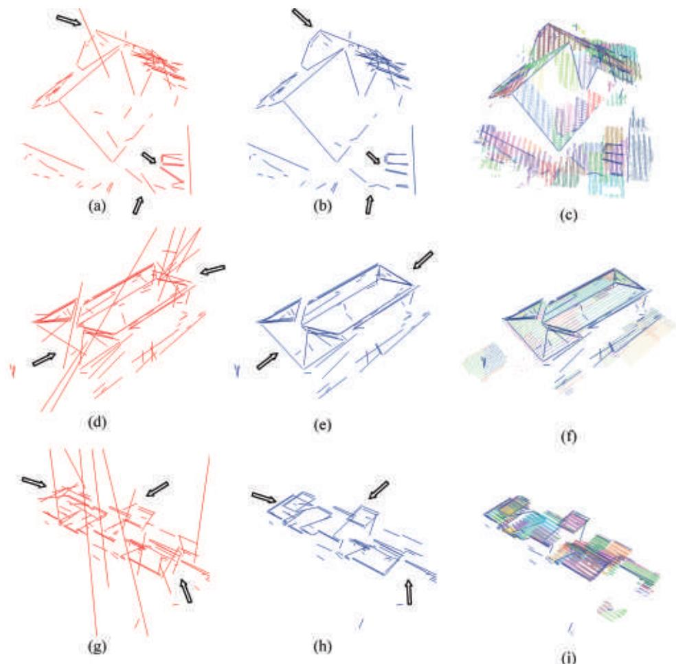
**Fig. 8:** 3D line segments generated with the method of direct construction (a, d, g) and our approach (b, e, h). Block arrows point to parts where some of the critical improvements are observed. The lidar point cloud overlaid with the lines reconstructed with our approach (c, f, i). Each colour in the point cloud belongs to the automatically extracted 3D planes in the vicinity of each line.
