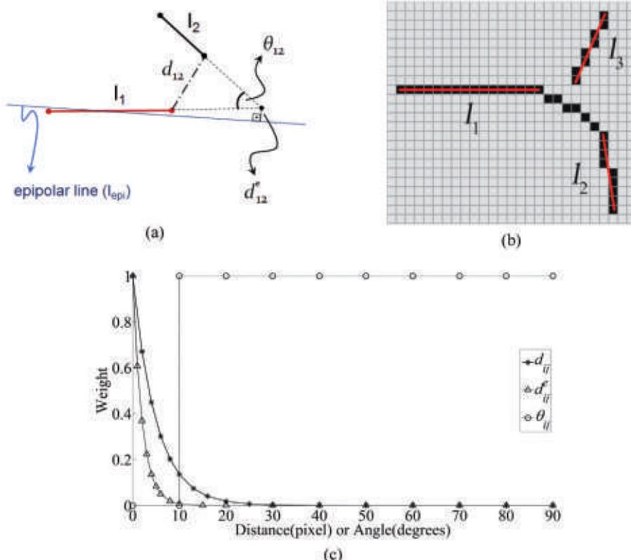
**Fig.5:** (a) Three measures used in the weight function, (b) the computation of minimum 2D distances in image space, and (c) independent weight curves for each measure. The control parameters are utilized as  $\sigma_1 = 5$  and  $\sigma_2 = 2$ .
