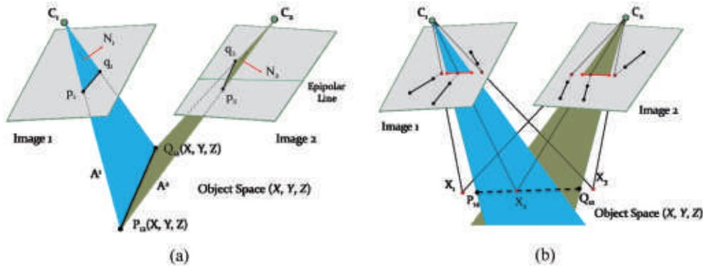
**Fig. 3:** The reconstruction of the line segments (a) that are not aligned with the epipolar line, and (b) that are nearly-aligned with the epipolar line. In (b), a dashed line style is used to illustrate that the line segment in object space is between the two projection planes.
