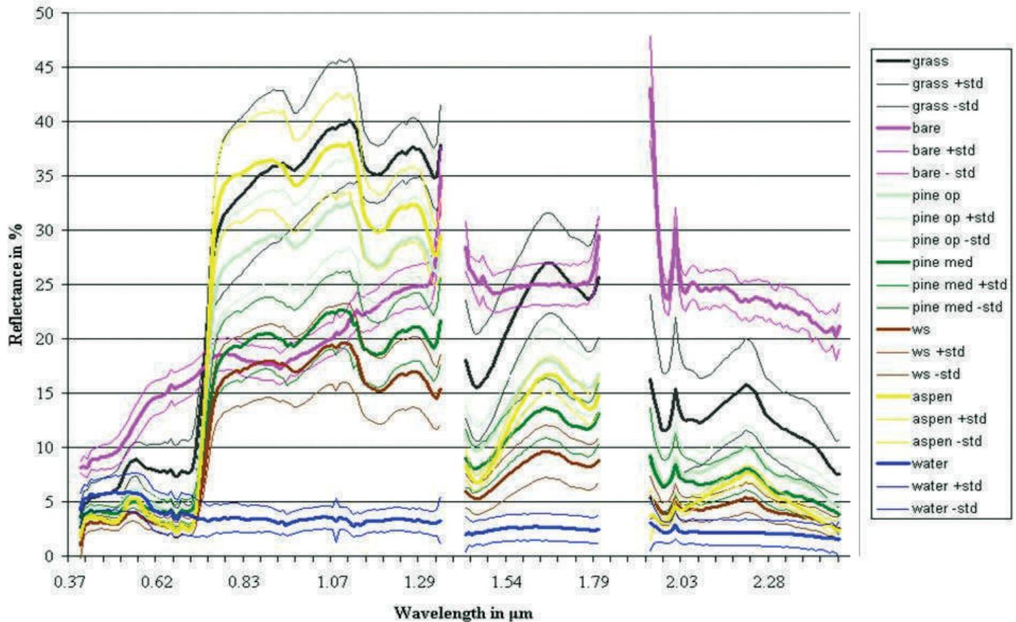
**Fig. 2:** AVIRIS spectra and standard deviation for land cover classes. The following AVIRIS bands were removed: 374 nm–394 nm (bands 1–3), 1354 nm–1424 nm (bands 107–114), 1812 nm–1951 nm (bands 153–168), and 2489 nm–2509 nm (bands 222–224) because of strong atmospheric effects.
