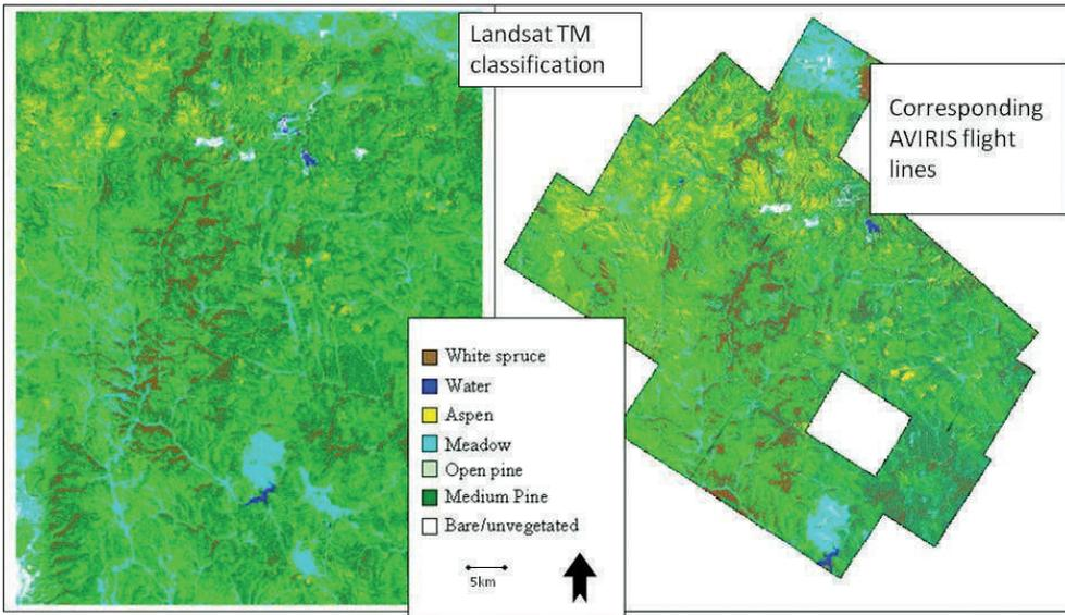
**Fig. 3:** a) Classification of combined spring-fall Landsat TM data (left) and b) AVIRIS classification (right). The missing scene contained errors that the data provider was unable to fix. No reference data was used from the area of the missing AVIRIS scene.
