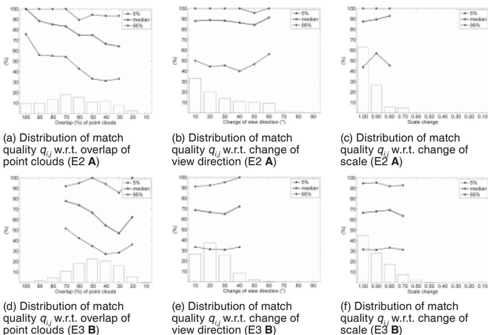
**Fig. 3:** The graphs show the dependency between the achieved match qualities  $q_{i,j}$  and the different sources influencing the matching. The bars at the bottom represent the relative frequency of the respective group. The lines in the graph represent the distribution of the grouped matching quality using the 5%, 95%-quantiles and the median. Groups with a relative frequency smaller than 5% are not considered.
