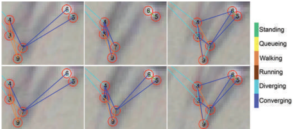
Fig. 5: Top: pedestrian interaction graph without HMM buffer; bottom: graph with HMM buffer.
