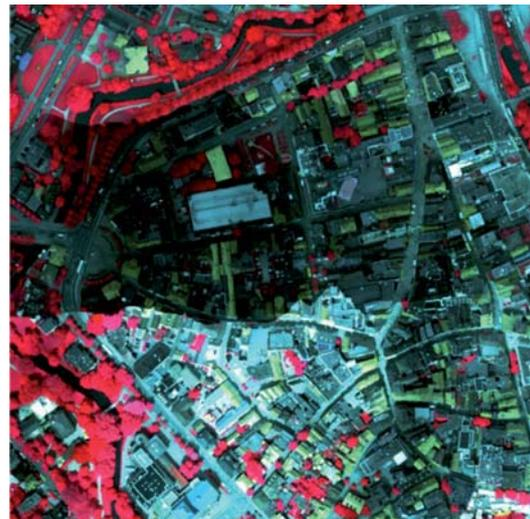
**Fig. 3:** A 500 m × 500 m subset of the pre-processed CIR reflectance image generated from three AISA+ strips. The spatial resolution is 50 cm. Note the sunny part of the lower strip compared to the other strips.
