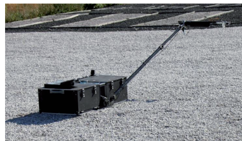
Fig. 3: The FIGIFIGO goniospectrometer measuring white gravel at the Sjäokulla test field.
