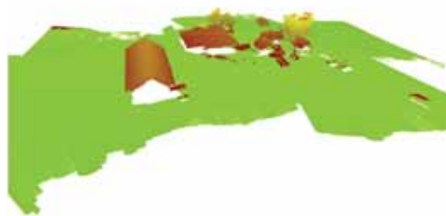
(a) Surface model generated from the lidar system.
