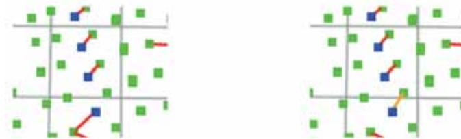
Fig. 10: Assigning point correspondences. Left: for every point of a 3D scan (blue), a corresponding map point (green) is initially assigned from the cell's point list (red line). Right: if the distance to neighbouring cells is smaller than the distance to the initial assignment, closer points might be found in the neighbouring cell (orange line).
