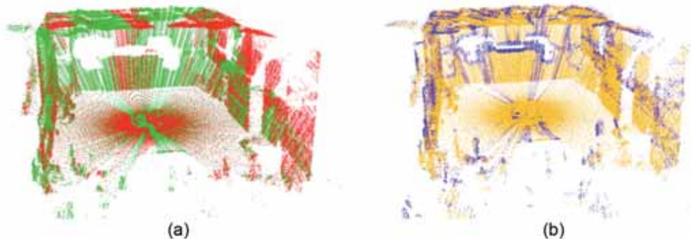
Fig. 6: Accumulated 3D scans of an indoor environment. (a) The colour encodes the different half rotations of the scanner. Moving the optical centre of the 2D laser range finder away from the rotation axis of the actuator results in different self-occlusions of the scans from the first (green) and the second (red) half rotation. (b) Measurements from first echo (yellow) and the second echo (purple). In case of partial occlusions, e.g. by the MAV itself, multi-echo detection leads to an increase of distance measurements.
