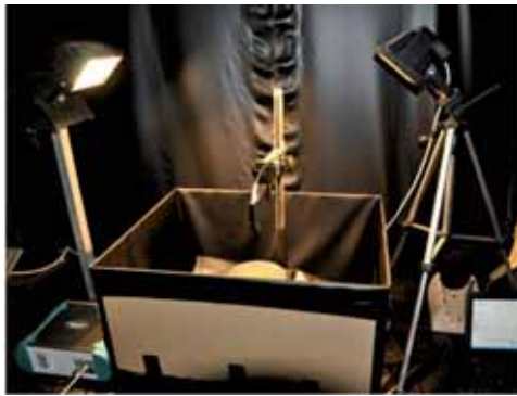
Fig. 4: Measurement setup with 8° fore optic. Two light sources at a distance of 50 cm illuminate the surface at 45°.
