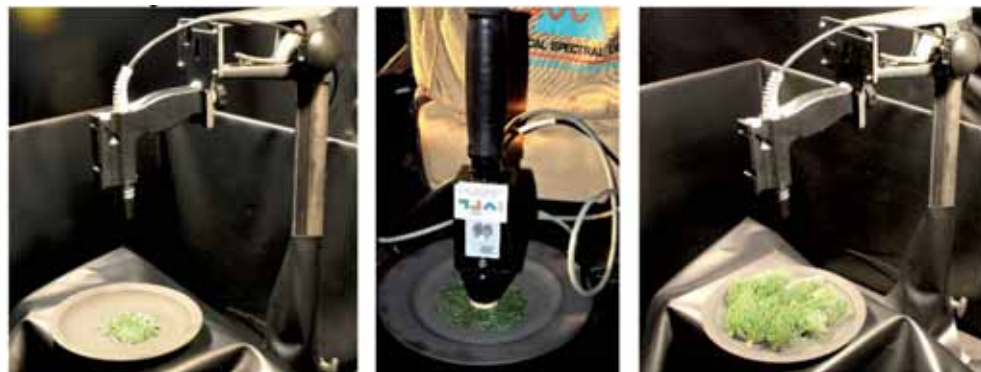
Fig. 5: Different spectra measurement methods: needles with fore optic (left), needles with contact probe (middle) and interlocking twigs (year 2012) with fore optic (right). Note that the light source is an integral part of the contact probe.
