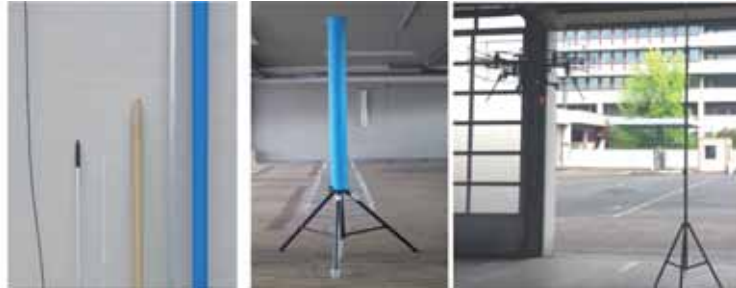
(a) Left: Six different object types, from left to right: cable (0.75 cm), aluminium broomstick (2.7 cm), plexiglass tube (5 cm), cardboard tube (7.5 cm), rectangular metal rod (4 cm), blue plastic tube (11 cm). Middle and right: experiment setup with object holder (black metal rod, 4 cm), measuring type and flying multicopter.
