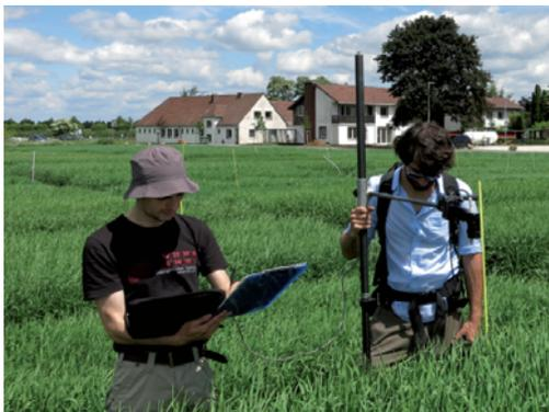
**Fig. 2:** Sampling hyperspectral ground truth with an ASD FieldSpec3.
