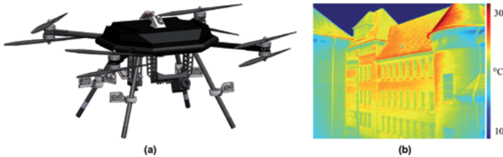
Fig. 1: (a) CAD model of an octocopter UAV sensor platform equipped with a thermal imaging camera FLIR A65. (b) Colour-coded thermal image of 640 pixel 512 pixel.
