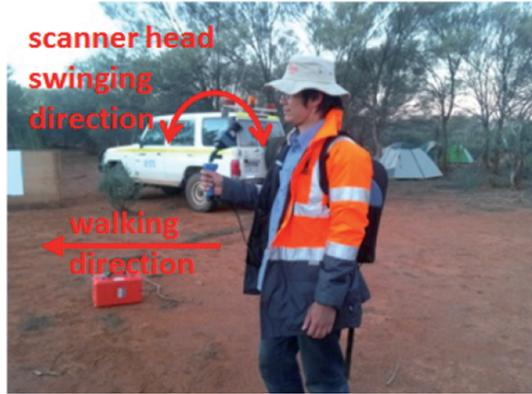
Fig. 2: Scanner head's and the user's motion.
