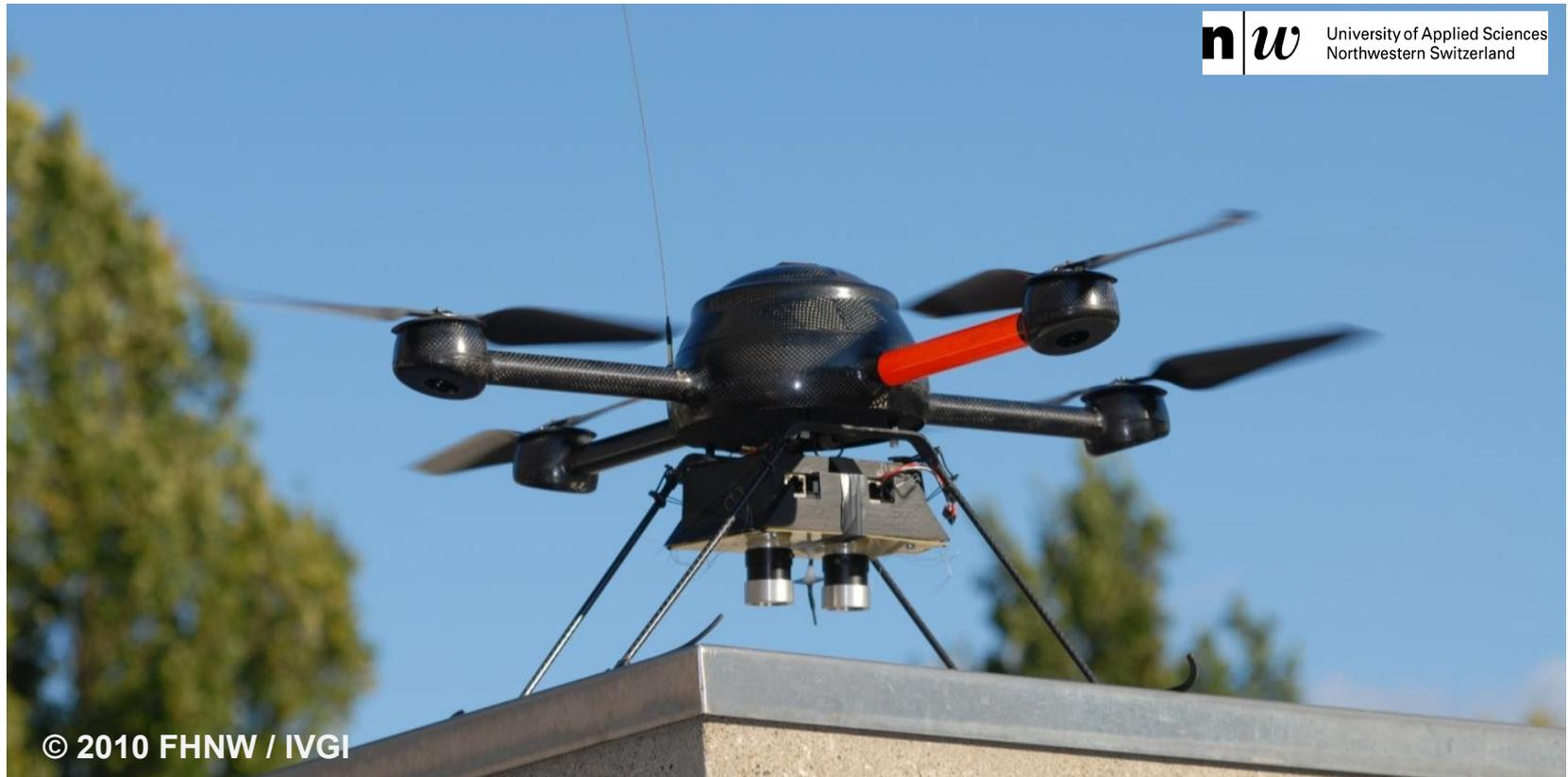
Prototype of light-weight multispectral sensor on microdrones md4-200
