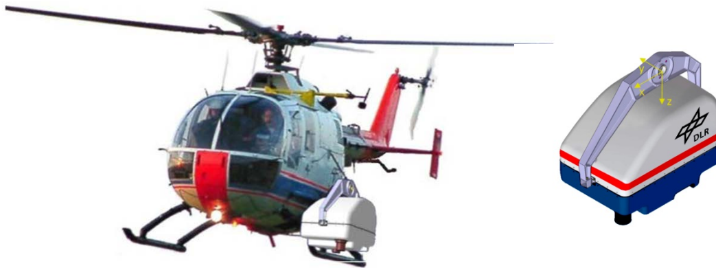
Fig. 1: 4k system mounted on the helicopter BO-105 (Simulation)
