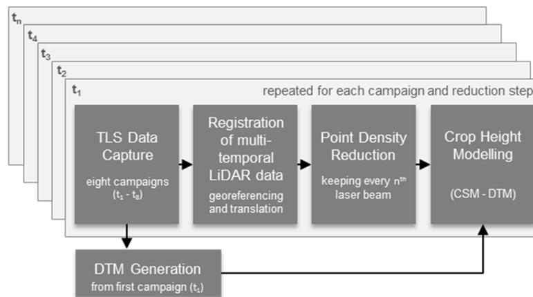
Fig. 3: Workflow of crop height model (CHM) generation from TLS data capture to CHMs calculation from reduced point density data sets.
