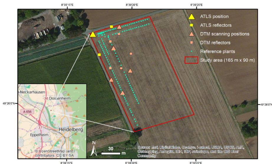
Fig. 2: Overview of measurement set-up located in Heidelberg (Germany) for simulation of autonomously operating terrestrial laser scanner (ATLS). Since the first campaign ( $t_1$ ) aimed to gain data for a complete high-resolution digital terrain model (DTM), multiple scanning positions and reflectors were used. For the subsequent set-up of the simulated ATLS system ( $t_2 - t_8$ ), only one scan position and two reflectors were used.
