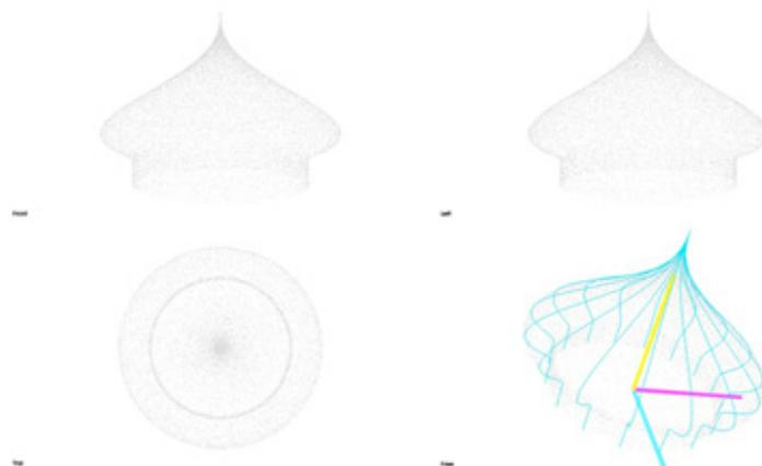
Fig. 6: Reconstructed profile curve from point cloud
