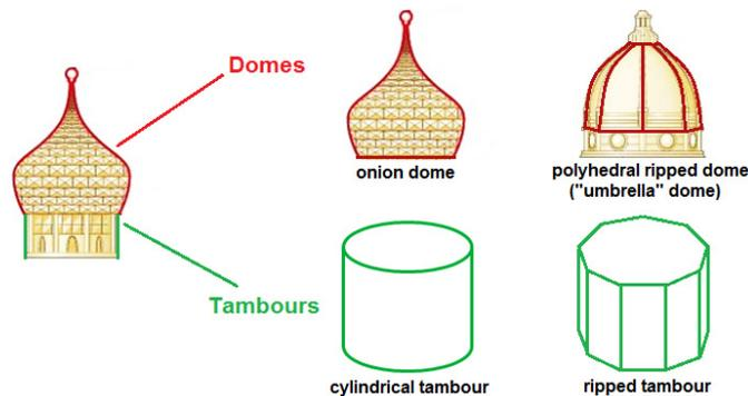
Fig. 2: Different types of domes and tambours
