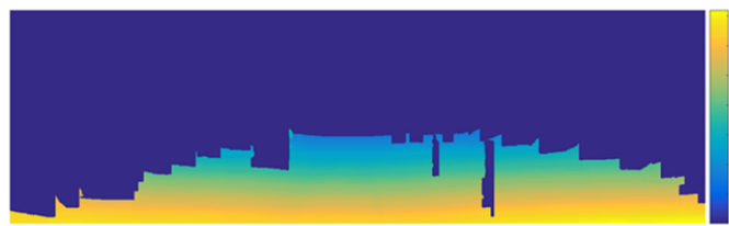
Fig. 5: The disparity map without vertical objects in the obstacle mask O_{mask1} (Fig. 2.a).
