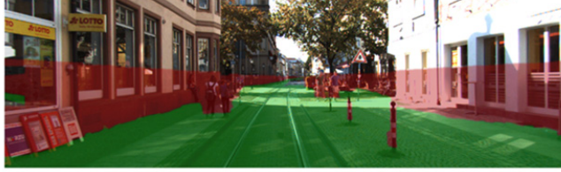
Fig. 6: Extracted ground plane (green) and areas of interest (red) in the reference image of a stereo pair.
