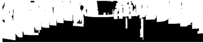
Fig. 3: The binary obstacle mask is built from the v-disparity image; obstacle pixels are shown in white.
