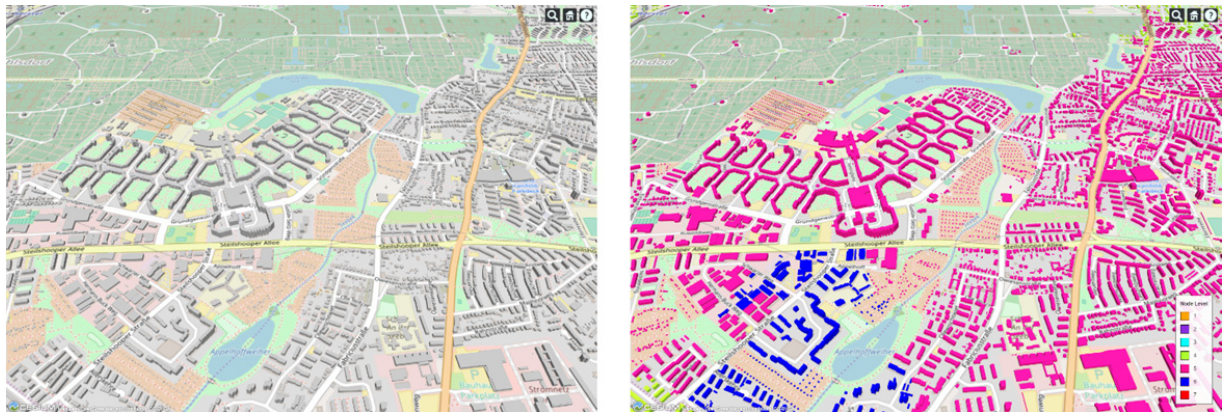
Fig. 9: I3S layer rendered in Cesium via the 3D Portrayal Service. On the left side the default style is used, on the right side the node level is used for styling
