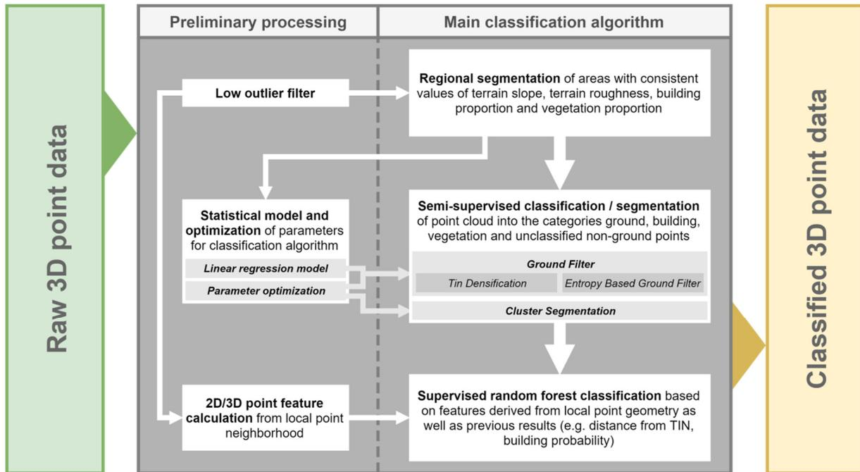
Fig. 1: Overview of the classification pipeline with the various processing modules grouped into preliminary processing modules and the main classification algorithm. Raw 3D point data is the input and semantically classified 3D point data the output of the pipeline.
