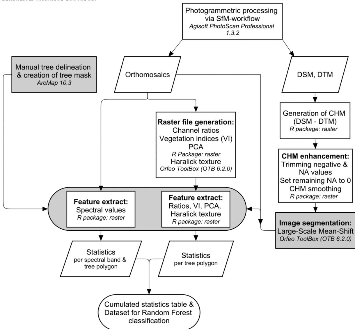
Fig. 2: OBIA workflow showing detailed steps of image data processing with reference to applied software packages
