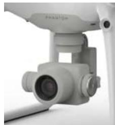
Sensor format  $13.2 \times 8.8\text{mm}^2$
